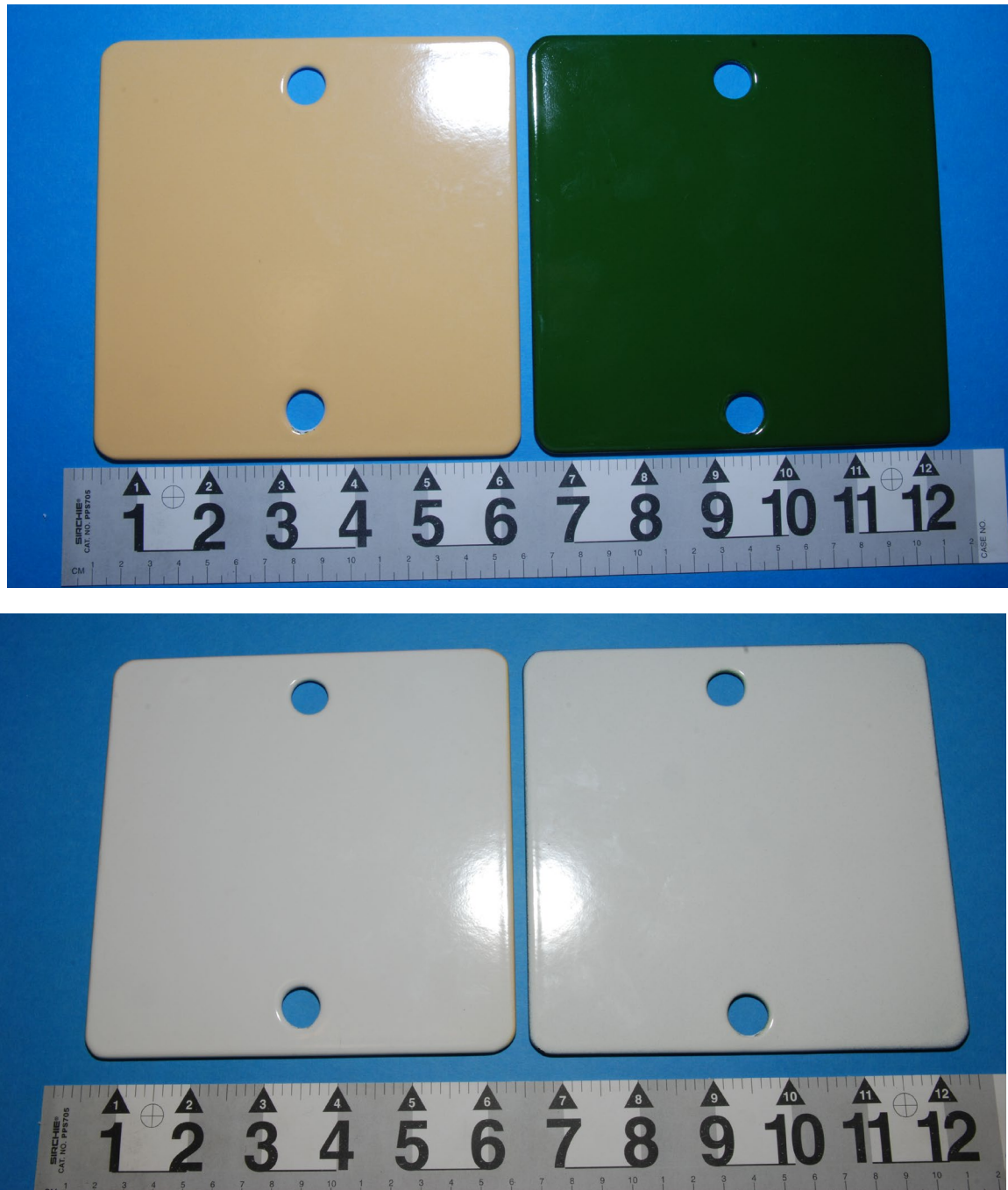
Figure 1 Image showing the colored side of the 6" x 6" glass-fused steel samples in the as-received condition.
